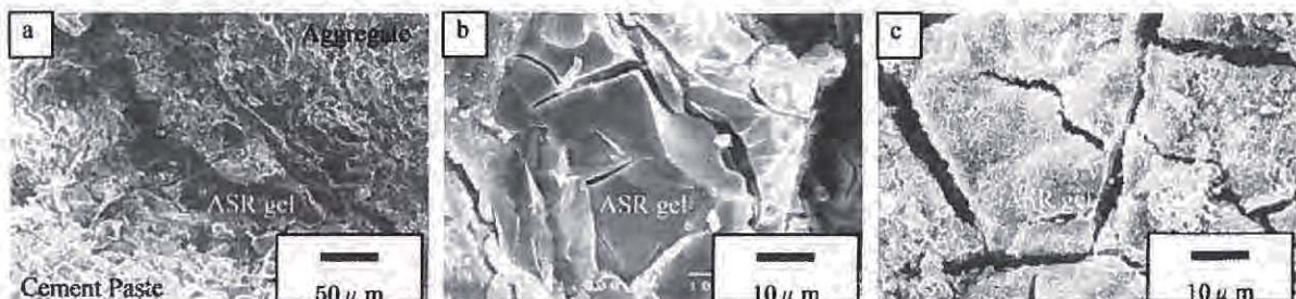
Fig. 5 SEM micrographs of ASR gel with Lithium ion : (a) Amorphous gel near an aggregate interface, (b) The enlargement of amorphous gel near an aggregate interface, (c) Gel whose surface is crystallizing near cement paste.
